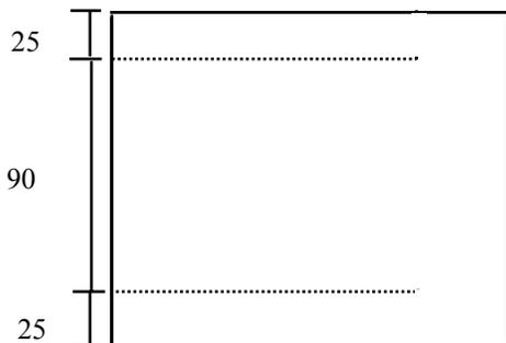
Fold along the two dotted lines to form the 25 mm shelf supports.
