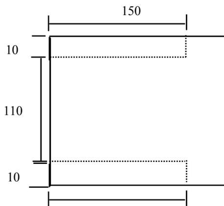
Cut along the dotted lines and remove the two 10 mm by 250 mm sections.
