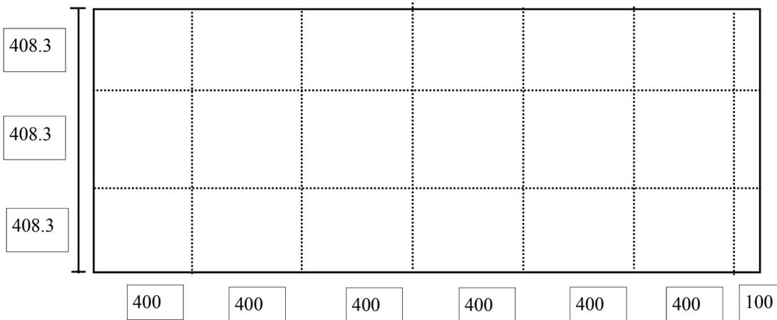
Take each piece and scribe the lines as shown but do **not** cut . Bend the 4 scribed lines to form a 4 -sided box with an 8 mm lip. See following page for a sketch of how the box should ap-
