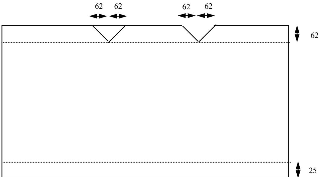
\*To make a crease , bend to 20 degrees and then flatten to remove the fold . When finished, the piece will lay flat with a small indentation
