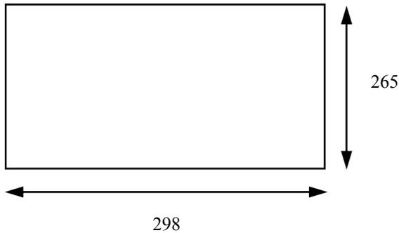
**2** Remove a 25 mm tab from each corner and then fold to form four lips
