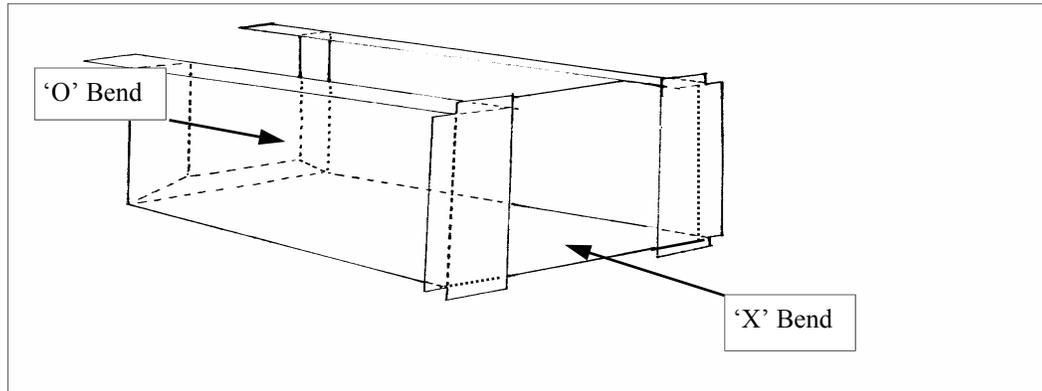
Place the oven jacket into the stove body and then slide the oven into Side panel 'B'/oven entrance.
