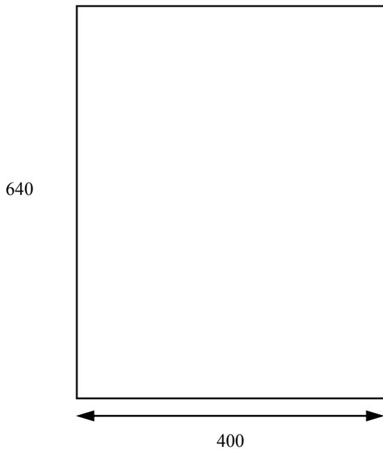
Remove a 25 mm tab from each corner and then fold to form four lips.
