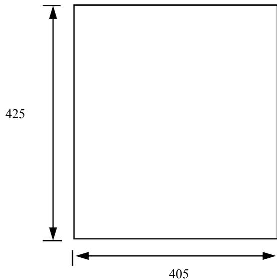
**2** Scribe and 'O' Bend two 25 mm flanges. Be sure to bend on the 425 mm side.
