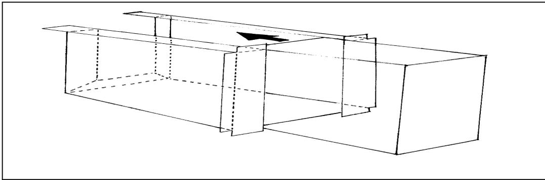
Use an arc welder to weld the **jacket** to the **oven** and the **jacket** to the **stove body**. The gap between the oven body and the jacket is important. See below for the proper gap on each side.
