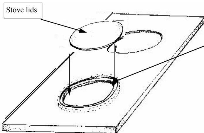
Once attached to the top plate, one half (or 5 mm) of the tubing should be visible from above. The exposed part of the square tube will form a lip that will support the stove lids. The stove lids can be used to seal the stove when the pots are not in place. This will keep smoke from entering the house.
