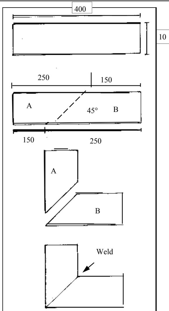
Take one piece of 100 mm by 6 metre square tube and cut a 400 mm section.
