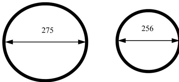
Bend each section into a circular ring and weld.
