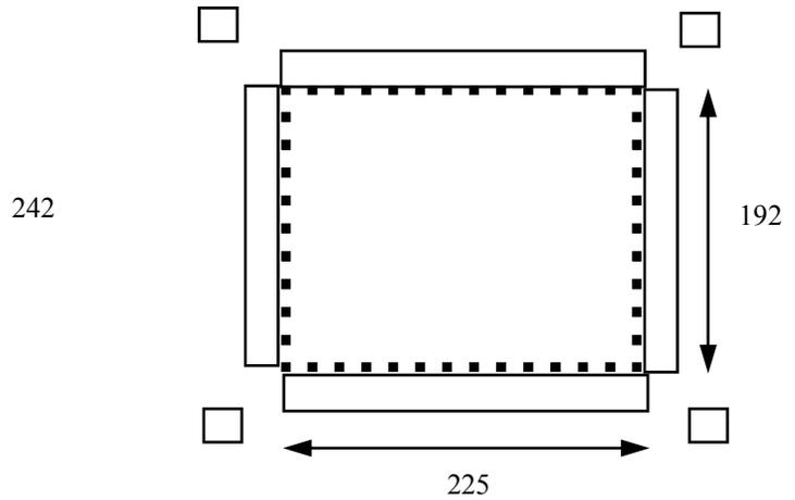
3 Insert the oven bottom into the **inside** of the oven box
