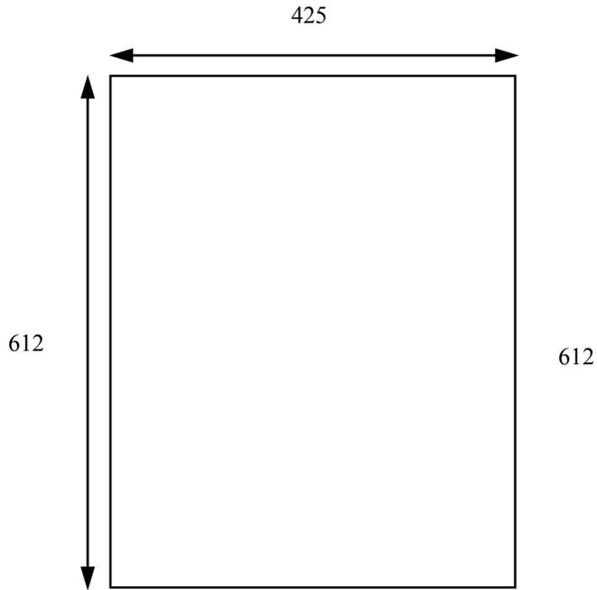
**2** Place the completed oven unit on the top right corner of the sheet—75 mm from the bottom and 55 mm from the side. Scribe but do not cut a line around the oven body.
