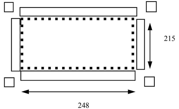
Fill the inside of the internal compartment with vermiculite or fiberglass insulation. Then weld the internal compartment to the inside of the external compartment. (**note: Be sure that the internal compartment fits into the oven before welding together.**)
