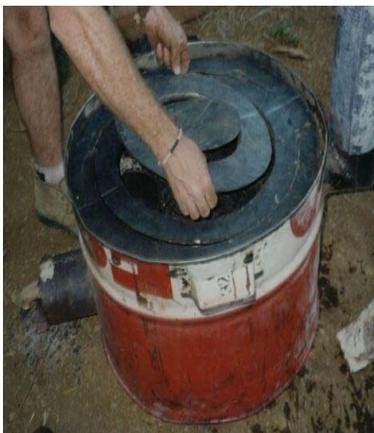
With the rings in place, multiple pots can be cooked at the same time. The rings can also be removed for use with individual round bottom pots.
