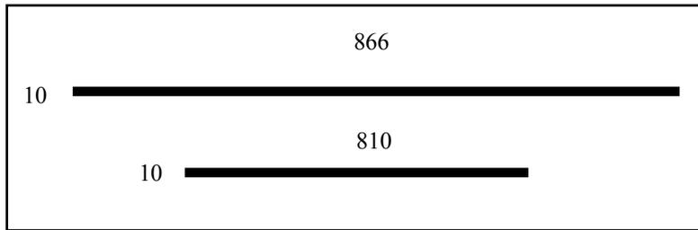
Take a piece of 2 mm by 10 mm square tubing and cut an 866 mm section and an 810 mm section.
