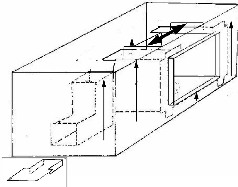
Insulation should also be added on top of the oven unit (between the
