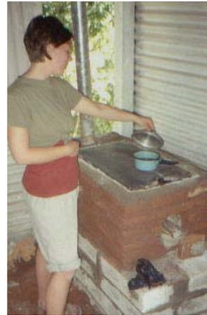
This brick stove –designed by Aprovecho - has an insulated rocket combustion chamber. Thousands of these stoves have been built in Central America. The metal lid is removable so a single pot can be cooked with direct flame.
