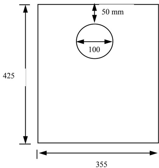
**4** Scribe a 95 mm circle inside the 100 mm circle. Cut the 95 mm circle and 'O' Bend the 5 mm flange to fit the chimney.
