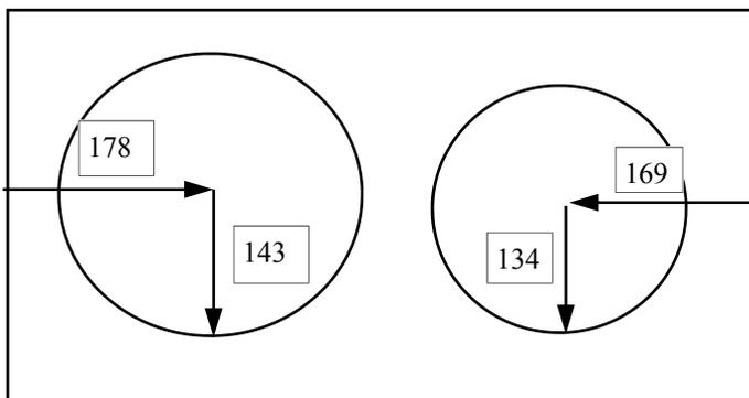
Scribe the large circle - 178 mm from the edge. Scribe the smaller circle -169 mm from the opposite edge. Use a jig saw or plasma cutter to cut the two circles. Try to cut the circles cleanly so that the remaining pieces can be reused as stove lids.
