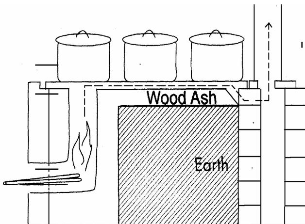
The type of material (cement ,brick , adobe or metal)) that is used for the exterior stove body will not have a great impact on the performance of the stove. Special materials are not needed for the stove *body*. The stove will function effectively as long as the body of the stove can support 5 pots and can withstand tempera-
