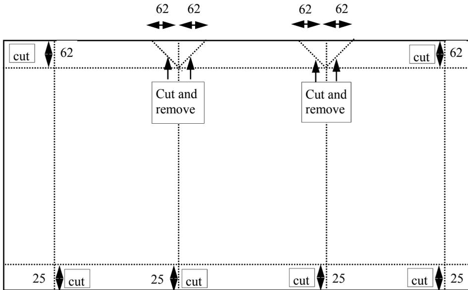
Make an 'O' crease\* along the 62 mm dotted horizontal line and then make an 'X' crease\* along the 25 mm dotted horizontal line. DO NOT FOLD.
