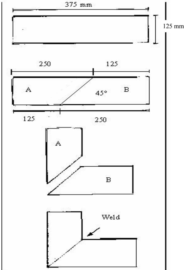
Take one piece of 125 mm by 6m round tube and cut one 375 mm section.
