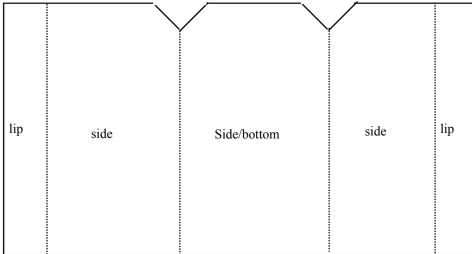
The jacket should now be a 3 sided box with two lips . Using the previous **crease** marks, fold an 62 mm 'O' bend and a 25 mm 'X' bend. Use pliers or vice grips to fold.
