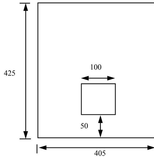
3 Scribe and cut a line 5 mm inset from the previous 100 mm scribe line. 'O' Bend the 5 mm flange to fit the perimeter of the combustion chamber.
