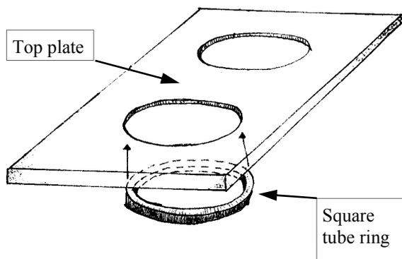
Take the top plate that you cut on the previous page and clamp it to the welding table (to prevent warping). Then tack weld the square tube rings to the underside of the top plate. note: although the drawing adjacent only shows one ring, be sure to attach both the front and the back ring. Attach the 275 mm ring under the large hole and the 256 mm ring under the smaller hole.
