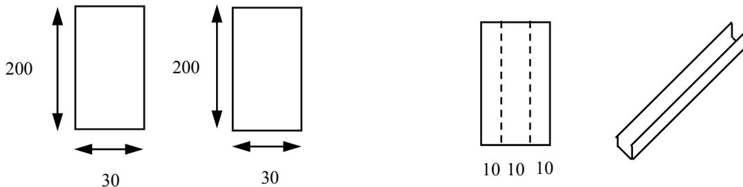
Place the top plate on the stove body so that the tracks enter into the oven jacket. Weld the 'tracks' to the inside of the skirt. The tracks should lay as close to the oven body as possible.
