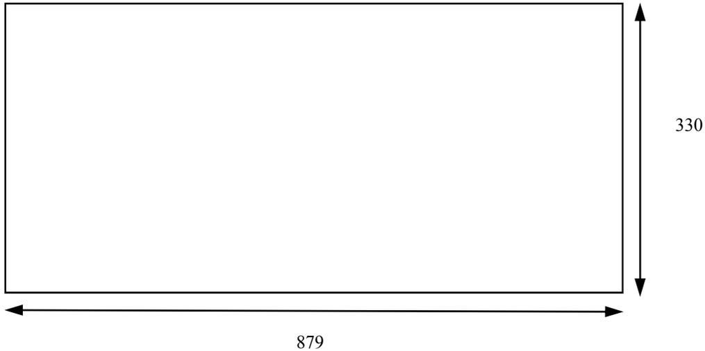
Scribe the lines as shown and then fold into a 4 sided box with a 25 mm lip. Weld with stainless steel welding rods. Before welding, double check that the 4 sides are exactly 25, 197, 230, 197, and 230.
