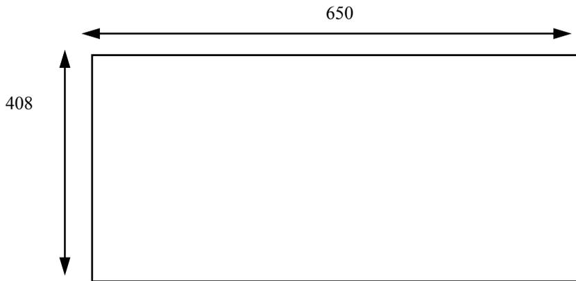
Take a piece of 2 mm mild steel and cut one 408 mm by 650 mm section.
