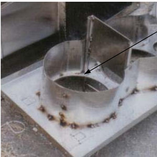
The top of the tracks - where the tracks meet the top plate - can be lightly pinched with vice grips to hold the damper in place when it is in the up (or closed) position . Be careful not to pinch the tracks too tightly or the damper will not slide at all.
