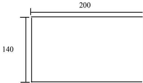
Cut one piece of mild steel or 3CR12 into a 200 mm by 140 mm section.
