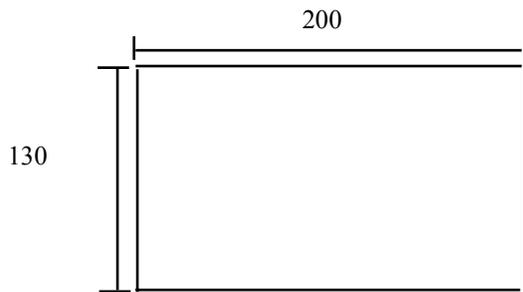
Cut one piece of 200 mm by 130 mm 3 mm mild steel or 1.2 mm 3CR12.
