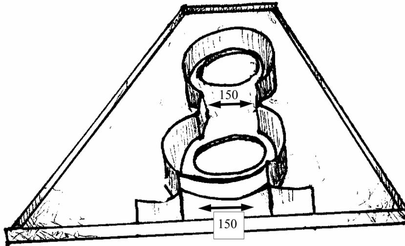
**Cutting the openings into the oven jacket.** **1 Oven Jacket entrance** Place the top plate/skirt unit on top of the stove body and A) scribe two lines where the bottom of the skirt meets the oven jacket. Then B) draw a third line joining the first two lines at the **front** of the oven jacket. Using an electric grinder cut these three lines. **2 Oven jacket exit** Repeat step A at the back of the oven exit. Then draw a third line joining the first two lines at the back of the oven jacket.
